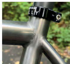
Top: Room for a mudguard or a bigger tyre. The fork crown port is for a dynamo cable Bottom: Welding as neat as I've seen on a titanium bike
