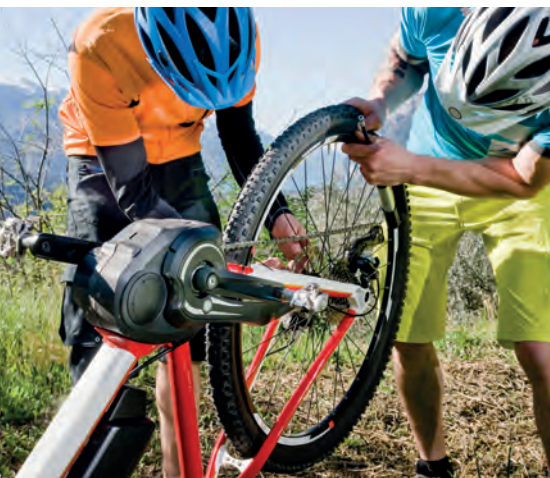
Above: Most e-bike maintenance jobs are the same as on a regular bike. Wheel removal is straightforward with a mid-drive as you don't disconnect a power cable to the hub Right: Any high-value bike, electric or otherwise, needs appropriate security. Heavy locks can be a drag to carry on a conventional bike but e-bikes make light of the extra weight
