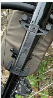
on rough terrain, even when loaded near their maximum weight of 3kg each and taken over foot-high drops. Their plastic frames were rock solid on the fork and the quickrelease mechanism kept the bags firmly in place.
