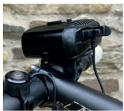
aero bar. There's an unsightly plate screwed to the top, which can be used with the contents of a 'Loaded' pack (available separately) to mount the light in front of and below a stem front cap. The light must not be strapped to the handlebar upside down, which would negate the cut-off beam feature.
