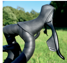
Above: The shifting isn't entirely wireless as the e-bike battery powers the rear mech
