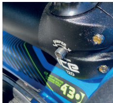
Top: A parking brake simplifies mounting and dismounting Bottom: A steering damper in the stem enables you to adjust the steering sensitivity
