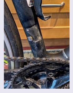
directly against the carbon fibre tube wall and can pull through if even lightly overstressed, weakening and enlarging the rivet holes. Assuming this is the case, the tube can be restored to full strength by a specialist repairer such as **carbonconcepts.co.uk**. **Richard Hallett**
