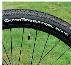
Top: Surly's slightly pricier cable discs are also decent Bottom: More spokes and wider tyres make off-tarmac touring more practical
