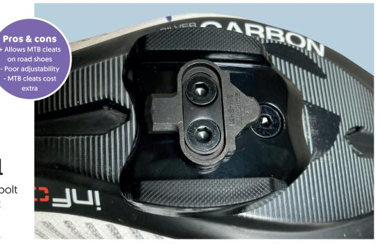
Shimano's Cleat Adapter SM-SH41 comprises, for each shoe: a triangular plate with a hole at each apex spaced to match the standard road threebolt fitting; three countersunk hex bolts to fix the plate to the road shoe sole; a moulded plastic block that fits over the plate; and a further two countersunk bolts to attach the two-bolt cleat (not provided) to
