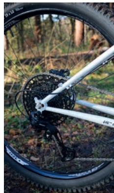
Those are 'Gnot-Boost' rear dropouts, spaced at 145mm. They'll fit 148 and 142mm hubs – or 135mm with adapters
