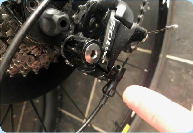
Rear/Right Hand Shifter Barrel Adjuster
