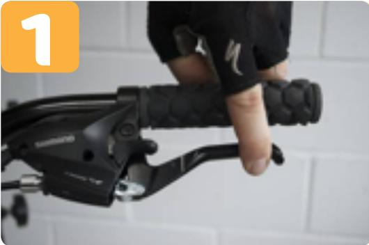
Shows the correct position of brake levers. Having the lever at the correct position is important, not only for safety but comfort and braking power. Your fingers are strongest with the fingers curled around the lever, however everyone has different sized hands and allowance should be made for this.
