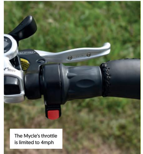
The Mycle's throttle is limited to 4mph
