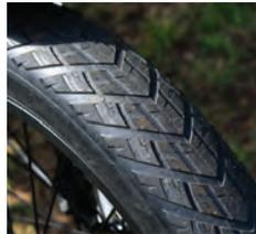
**Bottom:** 3in-wide tyres better isolate the load and rider from bumps and provide more traction when braking
